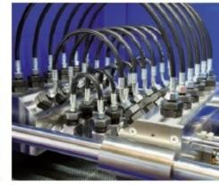
Pressure impulse test and hydrostatic testing in accordance with the common Standards, including flexing and half-omega Due to freely programmable pressure curves and axis movements, tests can be realized even beyond the Standards.
